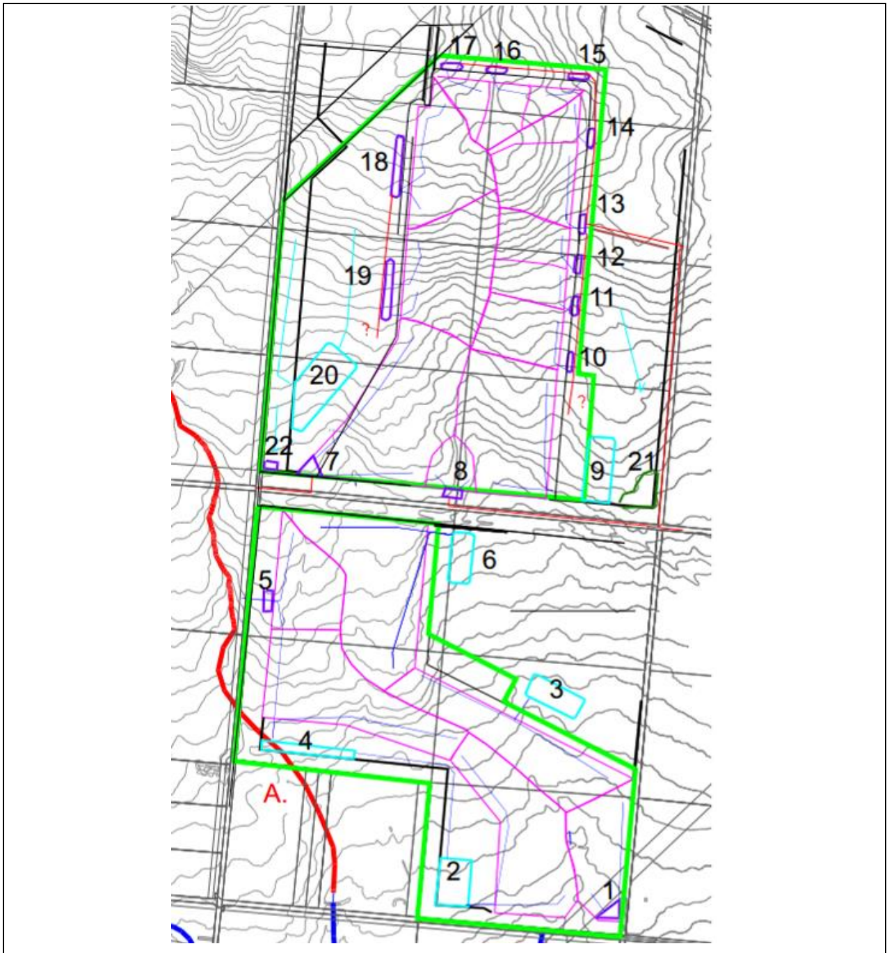
Figure 7 Site Stormwater Management Plan
